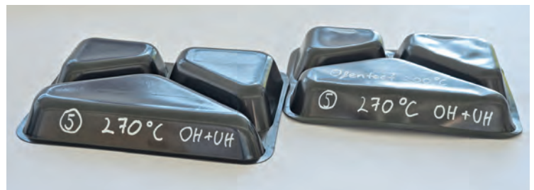
Figure 7. rCPET food trays made from material sheet 5 before and after the oven test at 270°C on upper and lower heater (© Illig)
