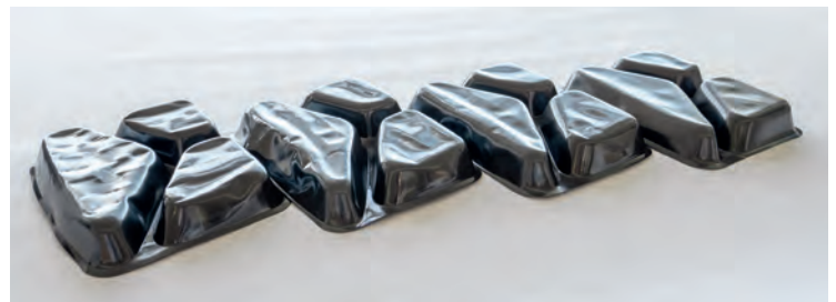
Figure 6. Oven tests at 200°C for 20 min: rCPET trays (from left to right: rolls 2, 3, 4, 5); upper heater at 250°C; upper and lower heating, lower heater at 270°C (© Illig)
