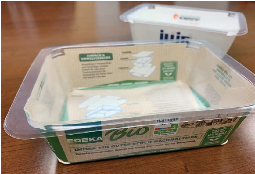
Demands from recyclers are driving increased adoption of packages where different materials can be easily separated.
